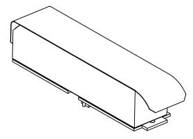
FIGURE 34: MICR Wiper assembly (part no. 7250601)
