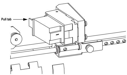
FIGURE 32: Cartridge removal
