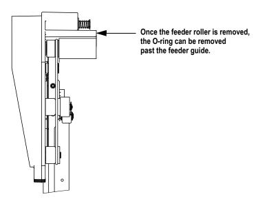
FIGURE 40: O-ring removal (Bird's eye view)
