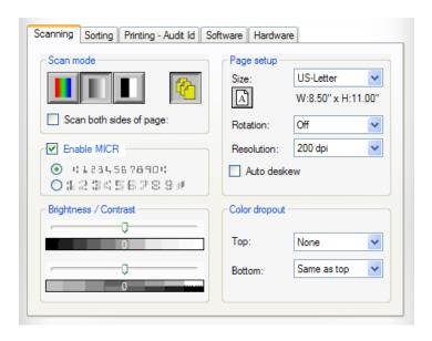
The scan mode settings determine which color mode the scanner will use, the desired feed mode and whether or not you want to scan both sides of pieces.
