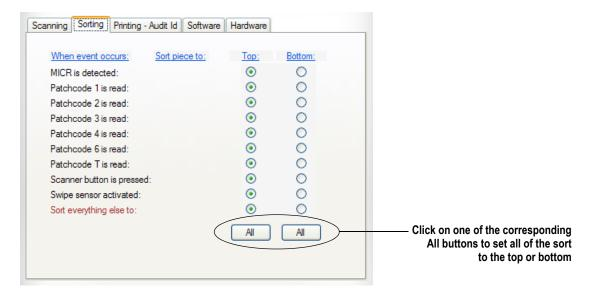
Set up the DS1225 to sort pieces to one bin or the other based on a particular event, such as when MICR ink is detected on a piece, or when the configurable Action (Scanner) button is pressed. For each event, select the top or bottom button, depending on how you want to sort pieces.
