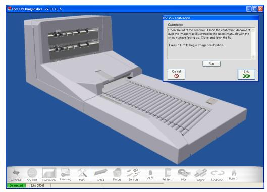
FIGURE 50: Standard Diagnostics - Calibration Wizard
