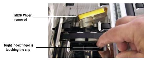
FIGURE 36: MICR Wiper removed
