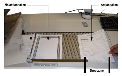
NOTE: If the drop zone is set as shown below, the action will be taken on the second piece, and NOT the piece you used to swipe the OpAssist sensor. In this case, the action is always applied to the next piece to enter the scanner.
