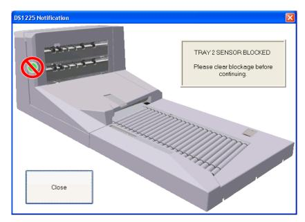
• BIN\_2\_PATH\_SENSOR\_BLOCKED\_JAM: The system had detected a blocked sensor for the top sort tray. Open the transport door to clear the jam.
