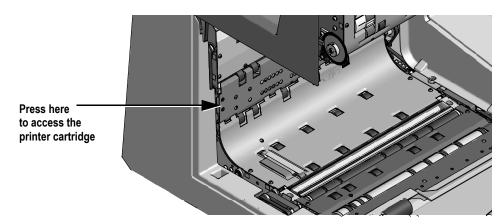
FIGURE 30: Opening the paper guide cover plate
