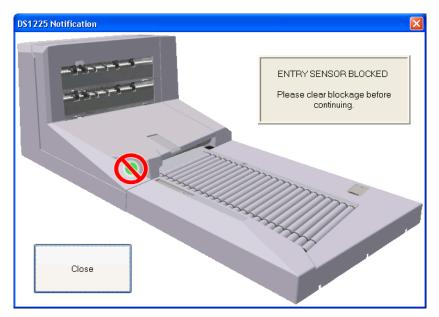
• **SYSTEM\_ENTRY\_SENSOR\_BLOCKED\_JAM**: The system has detected a covered system entry sensor. Open the transport door to clear the jam.
