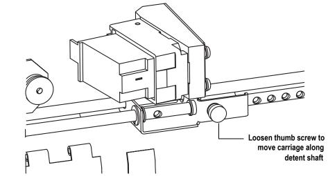
FIGURE 33: Adjusting printer position
