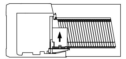
FIGURE 26: Clearing a jam
