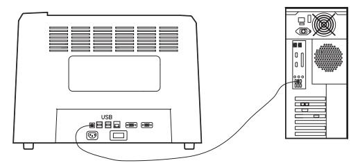
FIGURE 5: Connecting the DS1225 to the computer
