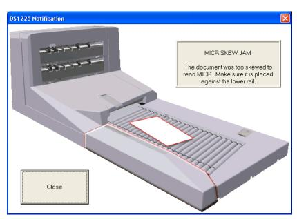
• MICR\_SKEW\_JAM: The system has detected that the item was too skewed to read the MICR line. Open the transport door to clear the jam, and place it against the lower rail before rerunning the item.
