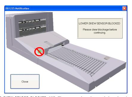
• LOWER\_SKEW\_SENSOR\_BLOCKED\_JAM: The system has detected that the piece dropped is skewed greater than two degrees. Open the transport door to clear the jam.
