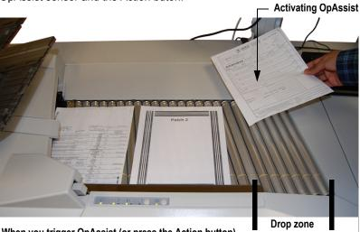
When you trigger OpAssist (or press the Action button) the scanner will apply the specified action for the piece dropped in the drop zone, not the pieces that are already on the track.
