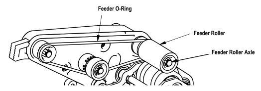
FIGURE 38: Feeder assembly O-ring location
