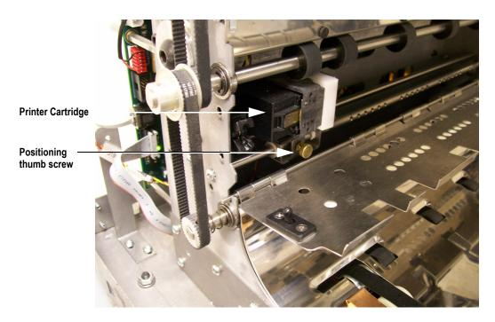
FIGURE 31: Accessing the printer cartridge
