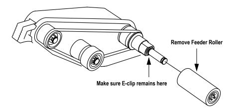
FIGURE 39: Removing the feed roller
