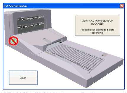
• VERTICAL\_TURN\_SENSOR\_BLOCKED\_JAM: The system has detected a covered vertical turn sensor. Vertical turn sensor is located prior to the sort bins. Open the transport door to clear the jam.
